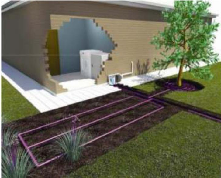
Using water from the washing machine and bathrooms, the Gflow automatically diverts, filters and disperses the water to the garden via a state of the art GF Drip line irrigation system. No need to ever move a sprayer around the garden again!
